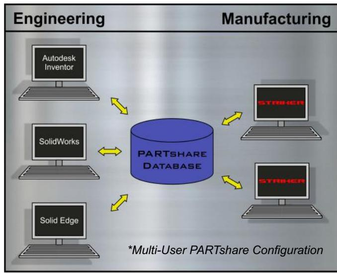
Parts placed into the PARTshare library from SolidWorks, Autodesk Inventor, or Solid Edge can be accessed by any of the STRIKER CAD/CAM and Nesting software modules. Parts can be retrieved individually for CNC processing, and SS-Nest also relies on the PARTshare library for nest job construction. This means parts placed into PARTshare from engineering are immediately available for nesting operations.
