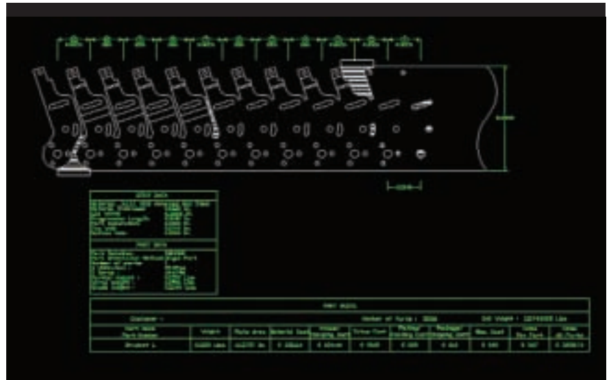
This dimensioned strip layout, a critical aspect of A.K. Stamping's die-design process, is created automatically in SS-Strip Design software.
